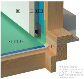
Figure 10 Marble floor tiles - Exterior deck
