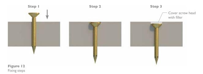
Screw to be covered up with filler before coating over it for aesthetic purposes and better protection against water ingress through screw points.
