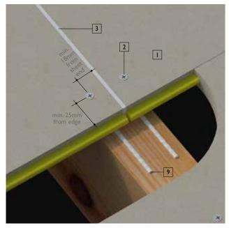
**Figure 4** Butt joints - Wet areas
