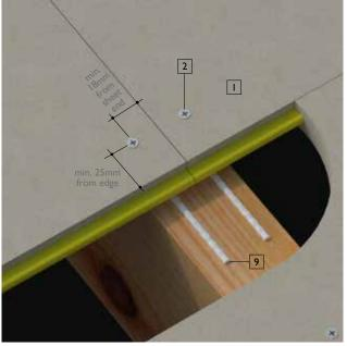
Figure 3 Butt joints - Internal dry areas
