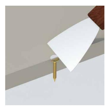
Figure 13 Sealing over fasteners (wet areas only)
