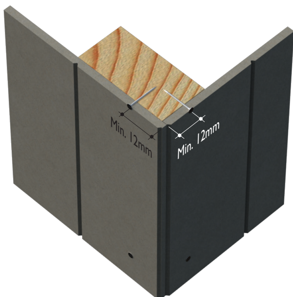
Figure 11 External corner joint
