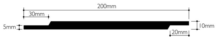
**KalsiPlank Interlocking section view**
